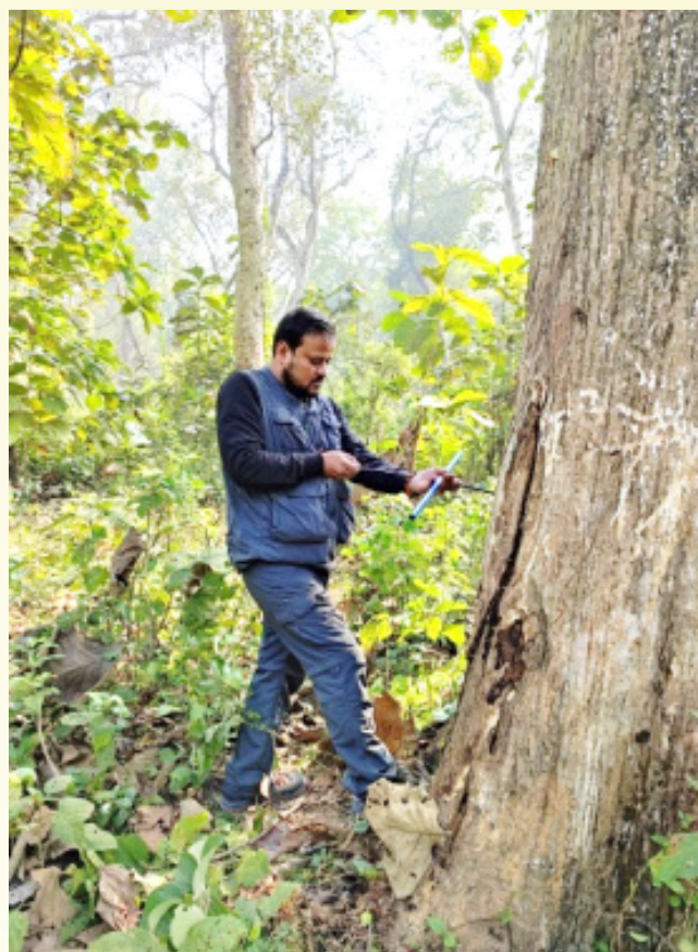
Sampling of tree-ring cores ( Tectona grandis ) from Maharajganj District, Uttar Pradesh, using an increment borer.
